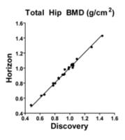
Figure 4. BMD correlation between Horizon and Discovery densitometers. Data courtesy of A. Myers and L. Jankowski. Illinois Bone and Joint Institute.
